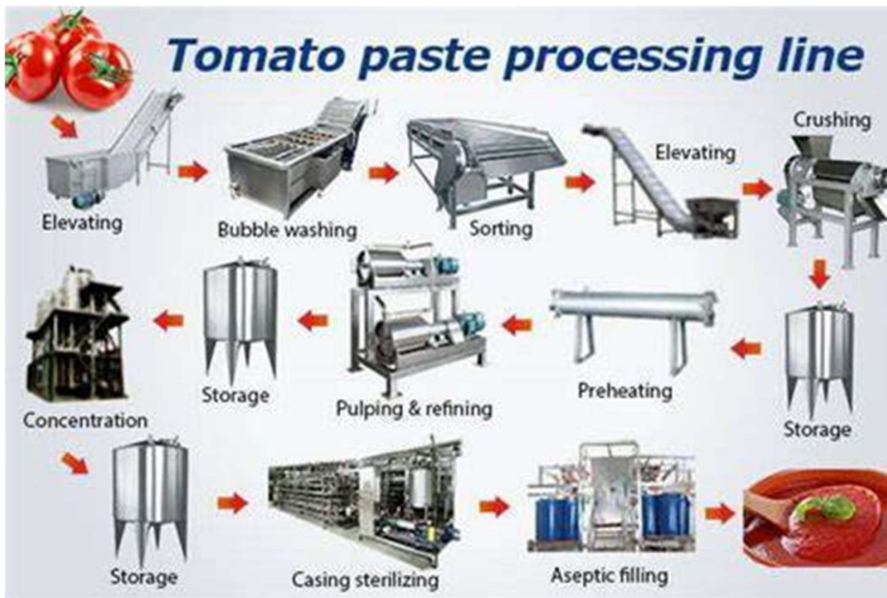
Figure: Flowchart of production of tomato-fruit puree / juice (from industry in Emilia-Romagna Region)
